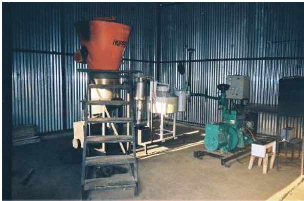
Figure 4.13: Biomass Gasifier set up in Madap-Thakarwadi, Taluka. Khalapur, District Raigad (Source: ARTI, 2012)
