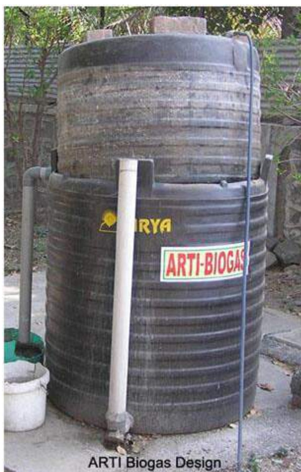
Figure 4.11: ARTI Biogasifier (Source: ARTI, 2012)
