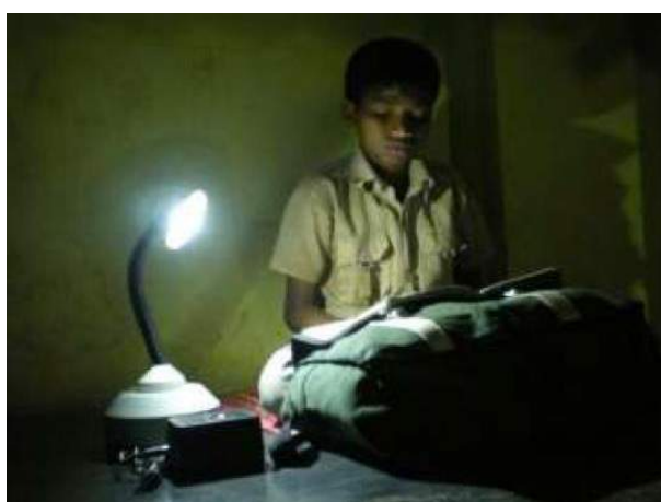
Figure 4.20: A child studying at night using a hi-power LED study lamp of approximately 0.5W total power consumption. (Source: Selco)
