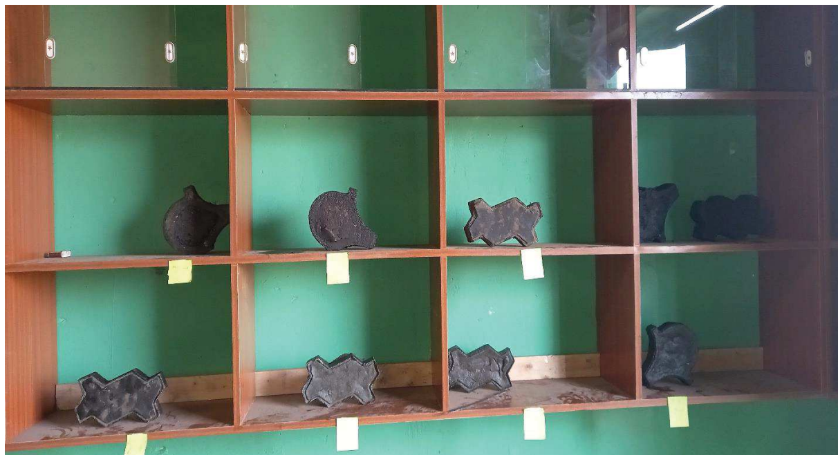
Image 13: Different designs of the pavement blocks produced by Chemolex Company from the Plastic waste
