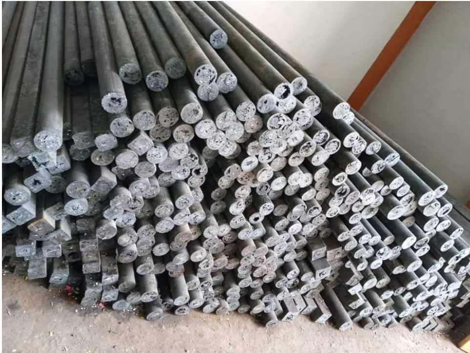
Image: Round Fencing Poles produced within the first week of the testing operation of the Extrusion machine.
