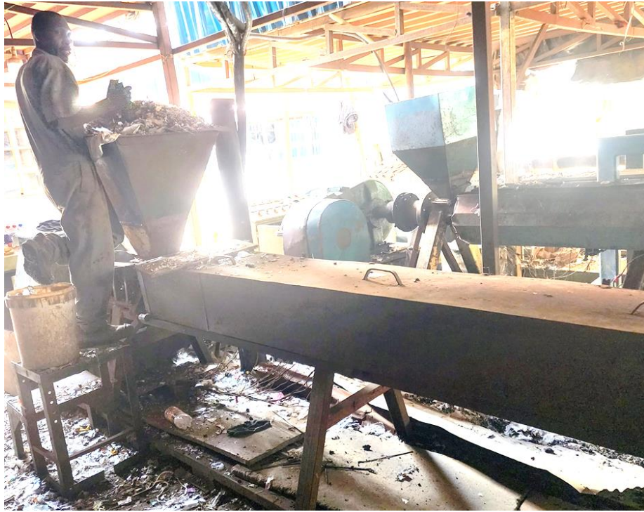
Image: Production of the fencing poles by utilizing the Extrusion machine
